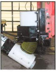
Picture shows hopper assembly mounted on a straight sided gravity box.
