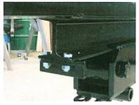
8: Insert hub & spindle assemblies into the spindle tubes on axle and fasten using ½" x 2½" bolts & lock nuts. Mount tires using wheel bolts. Determine which direction the toe-in is on the axle. Toe-in goes towards the lower frame tie bracket.
