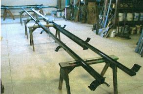
2: Assemble upper & lower plastic auger tubes using the tube connector. Make sure the connector flanges are pointing down. This will allow connection to sit in the lower support channel.
