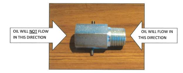
An in-line, pressure compensated, nonadjustable flow regulator value is available for CLOSED CENTER HYDRAULIC SYSTEMS. In the controlled direction, this regulator will maintain a constant flow rate of 10 GPM. This value should be installed on the pressure line, between the tractor and the value on motor. Thread is  $\frac{34''}{2}$  NPTF (must be reduced to  $\frac{12}{2}$ )
