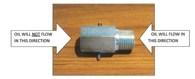
An in-line, pressure compensated, nonadjustable flow regulator valve is available for CLOSED CENTER HYDRAULIC SYSTEMS. In the controlled direction, this regulator will maintain a constant flow rate of 10 GPM. This valve should be installed on the pressure line, between the tractor and the valve on motor. Thread is  $\frac{3}{7}$  NPTF (must be reduced to  $\frac{1}{2}$ )
