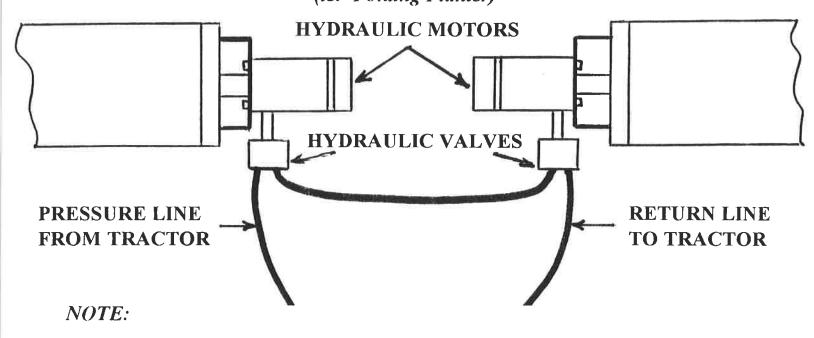
THE CROSSAUGER HYDRAULICS SHOULD BE CONNECTED INTO A SEPARATE SET OF REMOTES. IF THIS IS NOT POSSIBLE, THE CROSSAUGER MAY BE PLUMBED INTO THE PLANTERS EXISTING HYDRAULICS BY USING A MANUAL SELECTOR VALVE.
