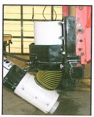
Picture shows hopper assembly mounted on a straight sided gravity box.
