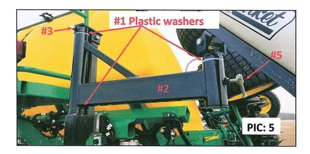
7: Remove cap and plastic washer from the top of the post. Slide the swing arm onto the post making sure not to damage the plastic sleeve. Re-attach the plastic washer and post cap. PIC: 5
