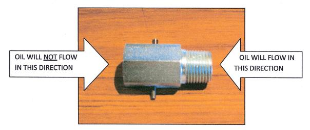
An in-line, pressure compensated, nonadjustable flow regulator valve is available for CLOSED CENTER HYDRAULIC SYSTEMS. In the controlled direction, this regulator will maintain a constant flow rate of 10 GPM. This valve should be installed on the pressure line, between the tractor and the valve on motor. Thread is ¾" NPTF (must be reduced to ½")
